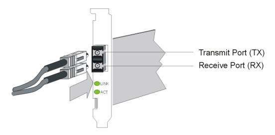
Figure 2. Connection of fiber-optic cables/plugs
